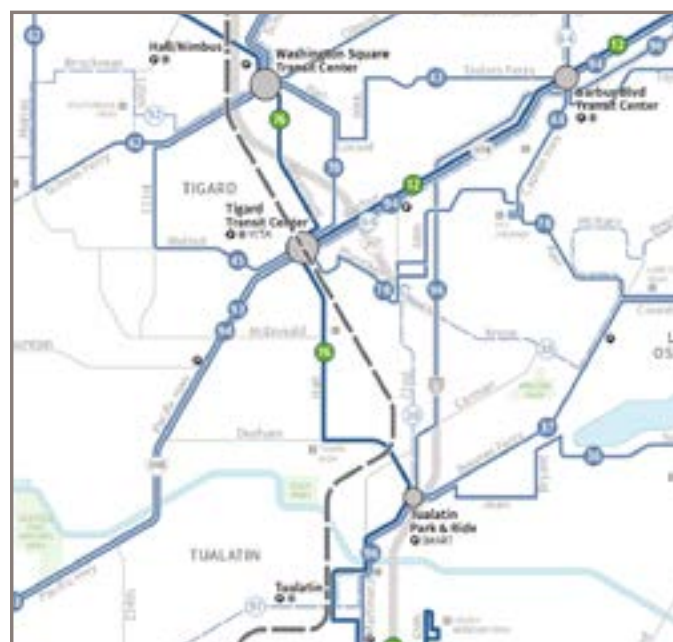
Figure 23: In areas where the development pattern creates obstacles to an efficient grid, routes converge on transit centers.
